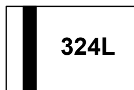
324L = Device Marking Code Bar denotes Cathode
